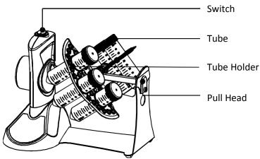
Before operating, turn the switch to "0" position, insert the tubes into the tube frame well. Turn the switch to "I" position. The instrument will start operating. Turn to "0" to stop operating. **Warning:**
