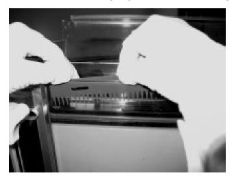
**13.** Using a pipette, softly load the sample solution into the well.
