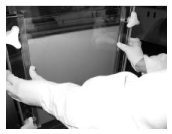
**9.** Fasten the four knobs in accordance with the direction
