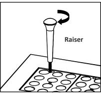
3. Lift the block up and out of the unit using the raiser tool
