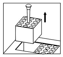
4. Remove the raiser from the current block, then secure it into the new block. Carefully place the block into the instrument.
