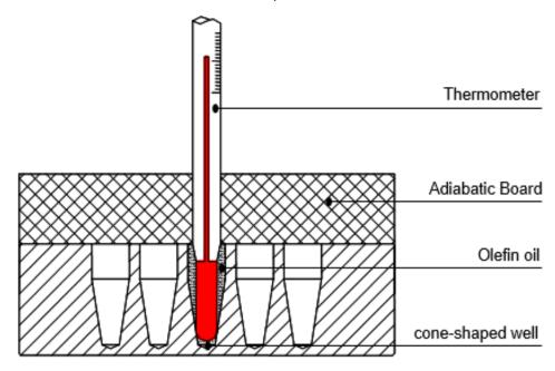
**NOTICE:** To ensure the calibration precision, read the actual temperature and allow 20 minutes for the temperature to reach calibration point
