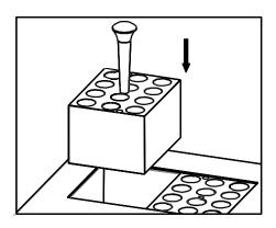
5. Use the allen wrench to fasten two screws into the block attaching it to the heating board, then remove the raiser.
