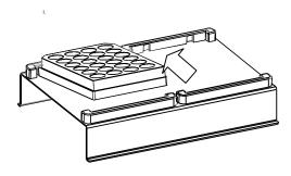
Hold the micro-plate up against one side of the edge of the stand (refer to above figure)
