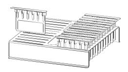
Vertically put the Gel card in the stand. One stand can hold max. 24 pieces of Gel cards. (Refer to above figure)
