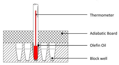
NOTICE: To ensure the calibration precision, read the actual temperature and allow 20 minutes for the temperature to reach calibration point.
