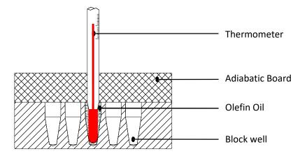
Press the up arrow and down arrow simultaneously under no operating status. The program turns to the right interface. The program auto controls temp. to 40 degrees C, an asterick displays and flickers. When it achieves 40 degrees C, cursor displays under decimal, "Adj" and asterick flicker together.
