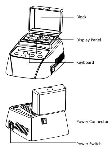
Turn on the power switch on the right side. The incubator runs the program to the setting temperature automatically. Heating always takes 15 minutes.
